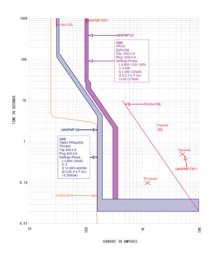
D. Over time the connected loads have changed from the original design, Q1 and Q2 circuit breakers are now simultaneously seeing a current flow of 140A.
