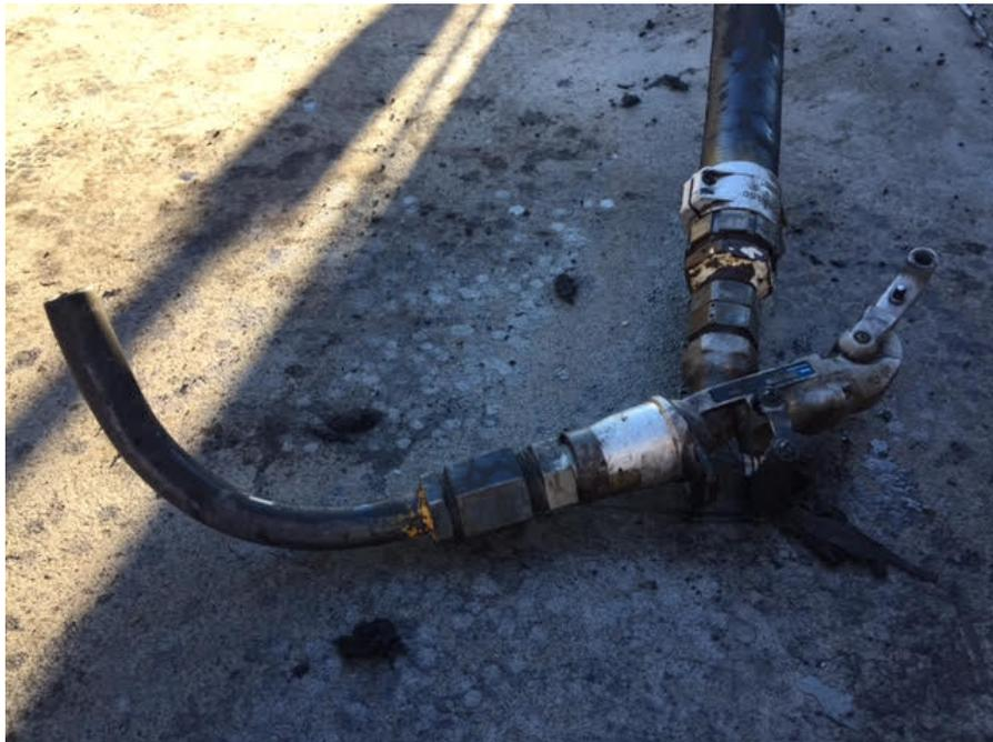
When attached the adaptor made a free-flowing nozzle that enabled plant to be refuelled without a quick connect coupling.
