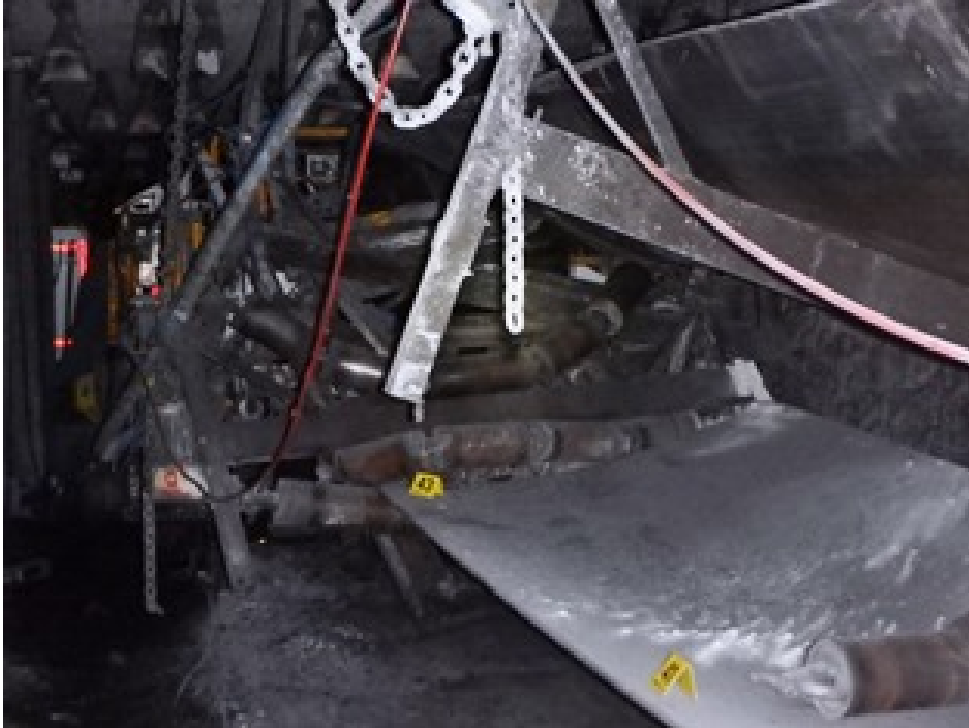
Figure 2: Failed connection hitch looking inbye at the DMU.
