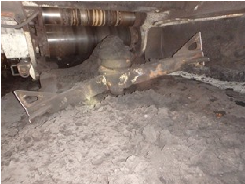
Figure 2: Failed connection hitch looking inbye at the DMU.
