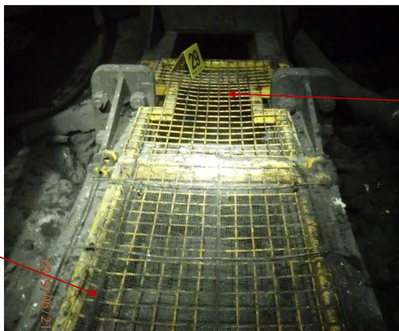
Reinforcement mesh overlaid by tech mesh on top of a fixed guard.
