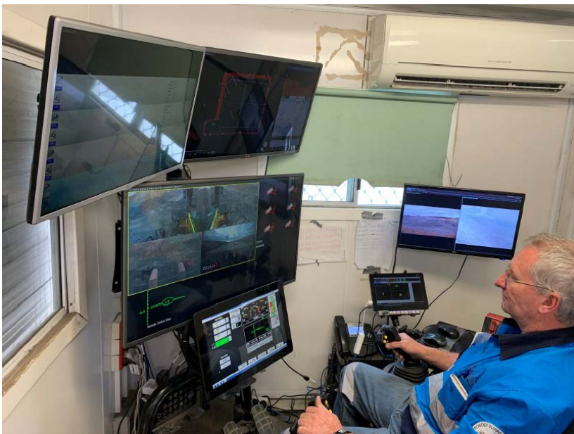
Figure 7 The remote operator station (ROS) inside the command for dozer control centre
