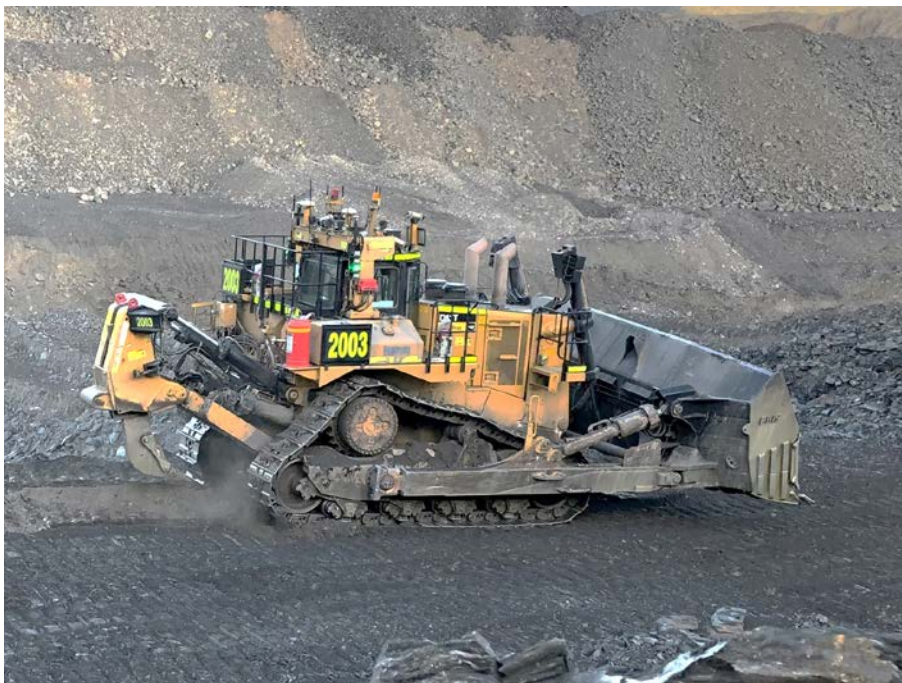
Figure 5 A dozer with modifications for semi-autonomous operations
