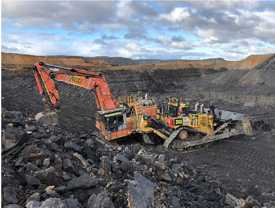
Figure 8 The incident scene immediately following the collision
