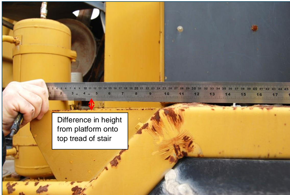
Figure 14: View from the platform of the top step tread to the lower steps. The outer edge flat bar welded stringer on the top stair tread is difficult to see.
