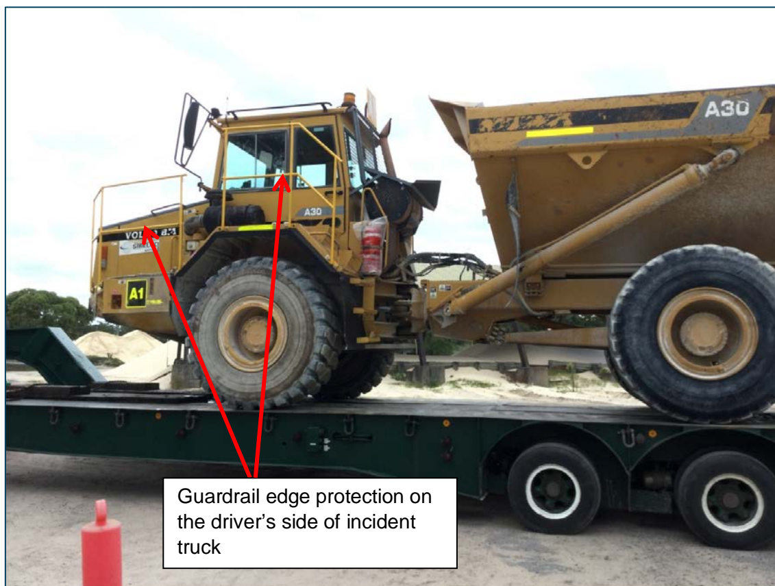
Figure 2: View from the driver's side access of the dump truck on the low loader truck on 1 February 2016. Note the two modified light yellow outer guardrails fitted to the walkway access areas on the driver's side of the truck.
