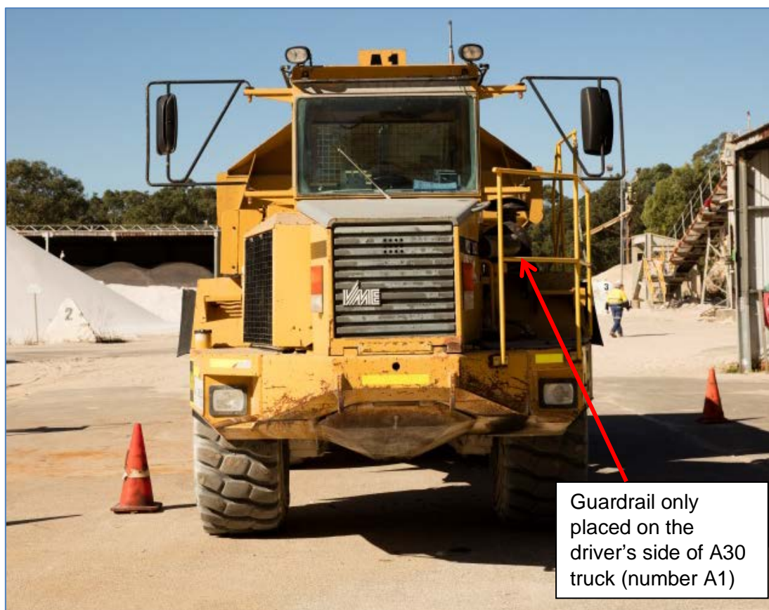
Figure 5: Front view of dump truck at Salt Ash site on 8 May 2016. Showing the modified guardrail fitted only placed on the driver's side platform.
