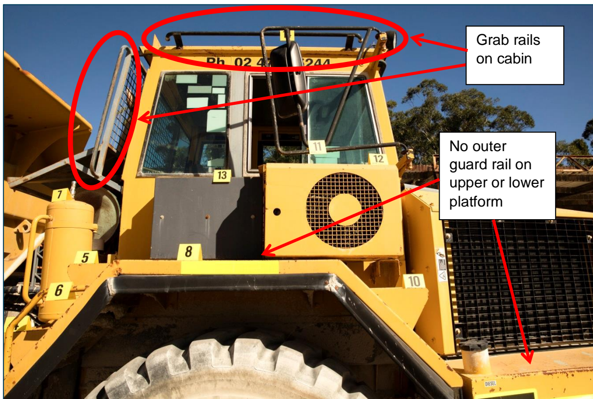
Figure 9: The hand hold and two grab rails on the truck. The vertical hand hold attached to the air tank, the near vertical grab rail attached to the cabin rear window guard frame and the horizontal grab rail attached to the top of the cabin. The photograph shows the wing mirror in a closed position. There is no guardrail on the outer edge of the upper or lower platform.
