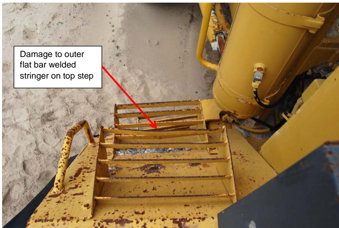
Figure 14: View from the platform of the top step tread to the lower steps. The outer edge flat bar welded stringer on the top stair tread is difficult to see.
