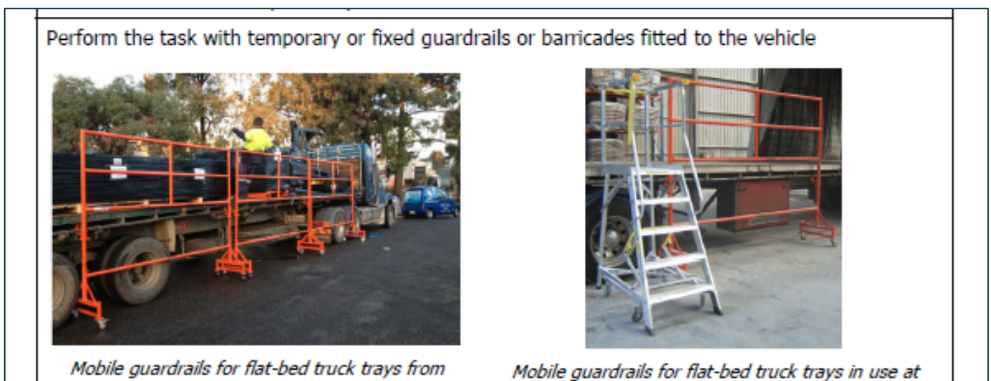
Figure 19: Extract from the Sibelco memorandum dated 23 June 2014, Controls for prevention of falls from vehicles . Examples of temporary or fixed guardrails or barricades fitted to mobile plant and use of mobile steps for access to mobile plant.
