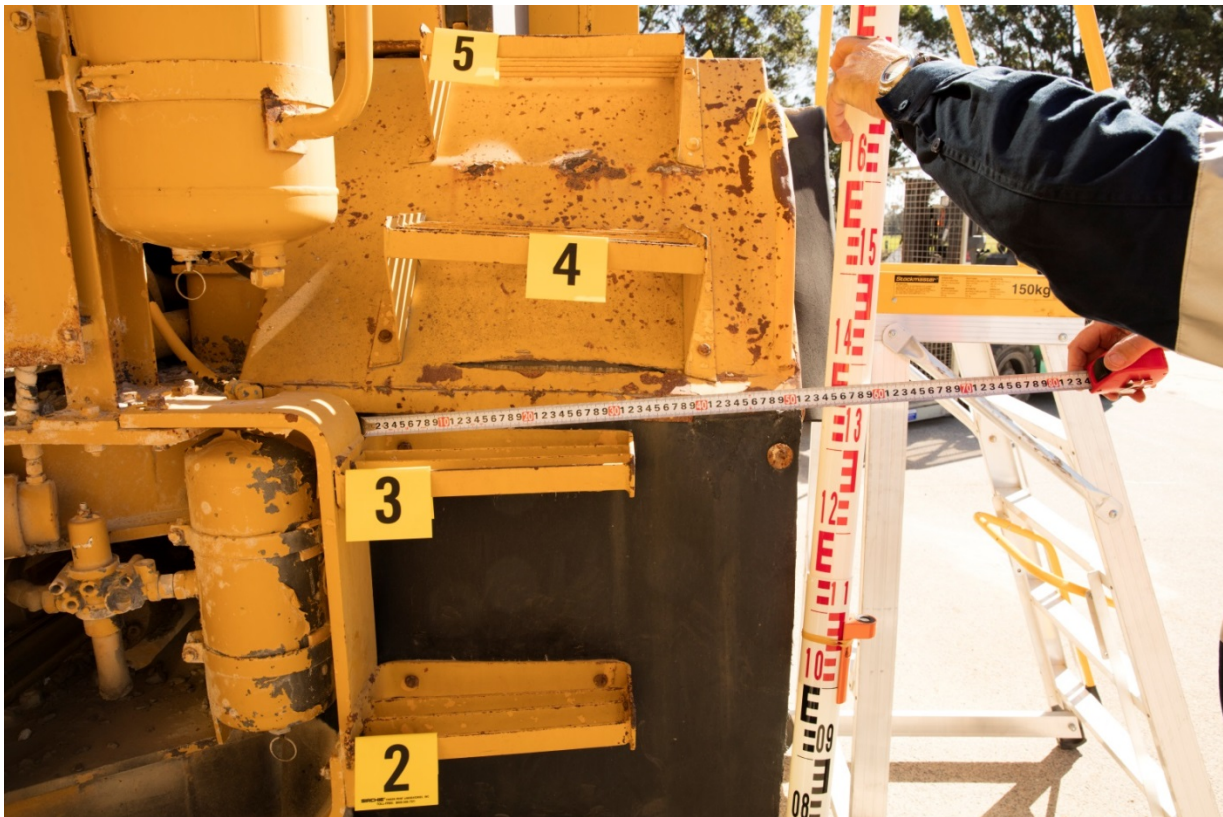
Figure 15: The narrower and offset step ladder rungs (number 2 and 3) leading onto the stair treads (number 4 and 5) on the off- side of the dump truck.
