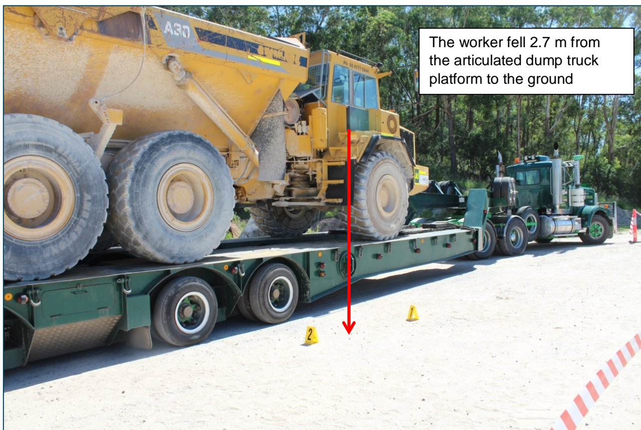
Figure 1: View from the right (off-driver's) side of the Volvo A30 A1 on the low loader truck on 1 February 2016. The two yellow numbered markers indicate the approximate location where the worker fell to the ground.
