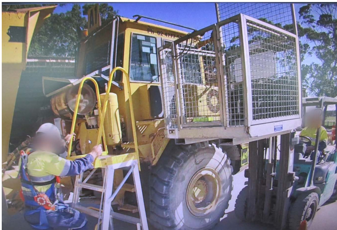
Figure 22: Access onto the dump truck platform using a mobile ladder and man cage.
