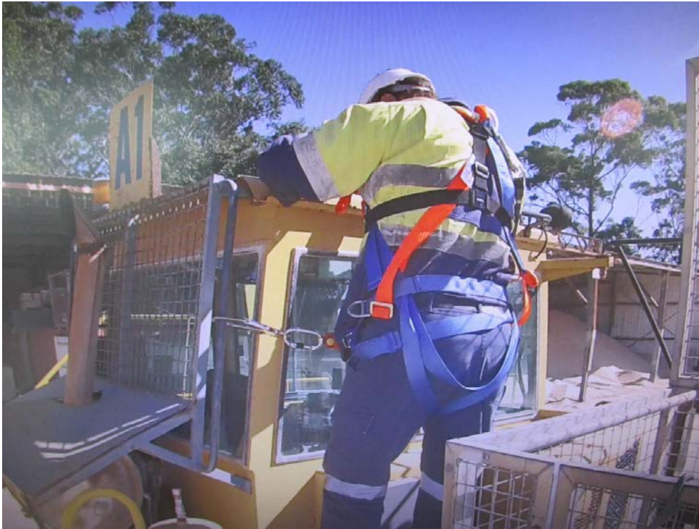
Figure 26: Person on the first stair tread and facing the stair looking for a right hand position to maintain three points of contact as they descend. Three points of contact is possible by first using the outer edge protection provided by the man cage and then the mobile ladder grab rail.
