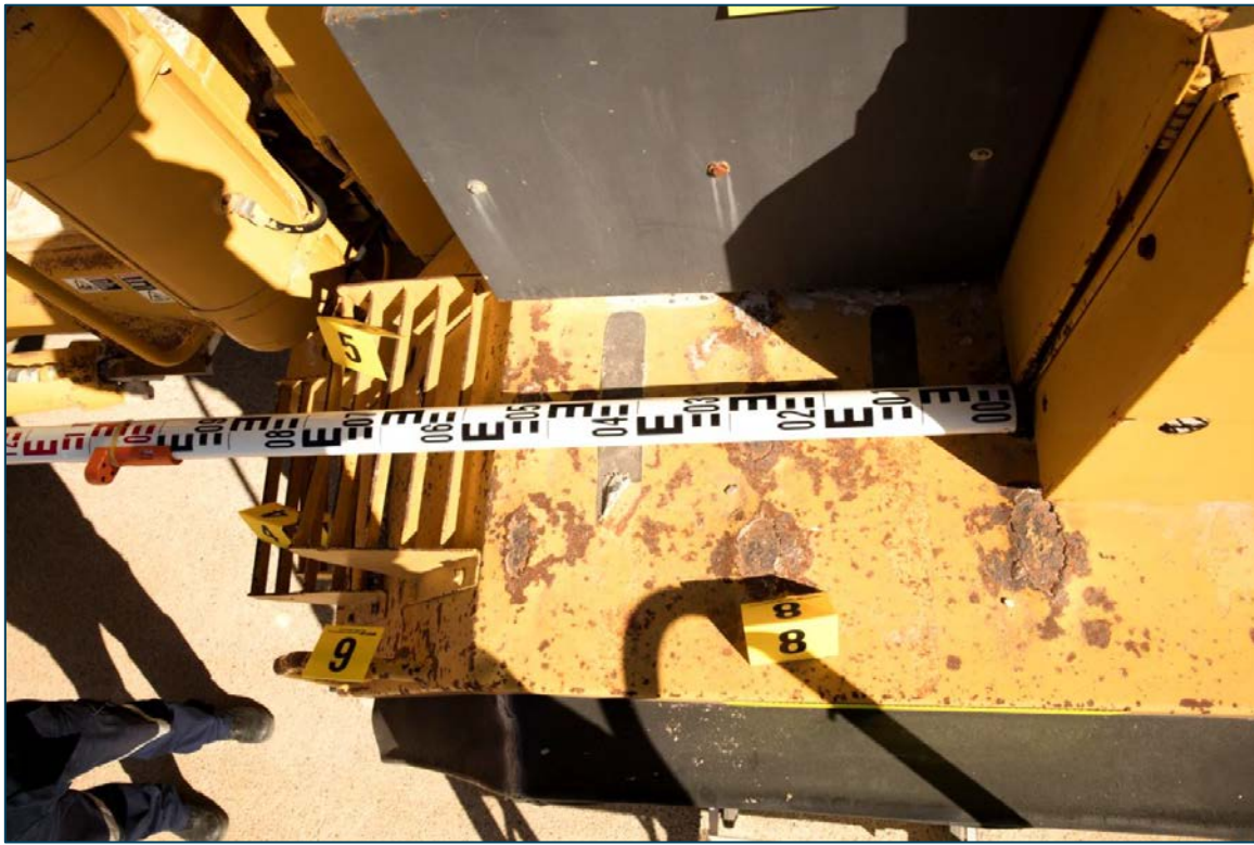
Figure 11: A closer view of the degraded condition of platform (position number 8) leading onto top of steps.
