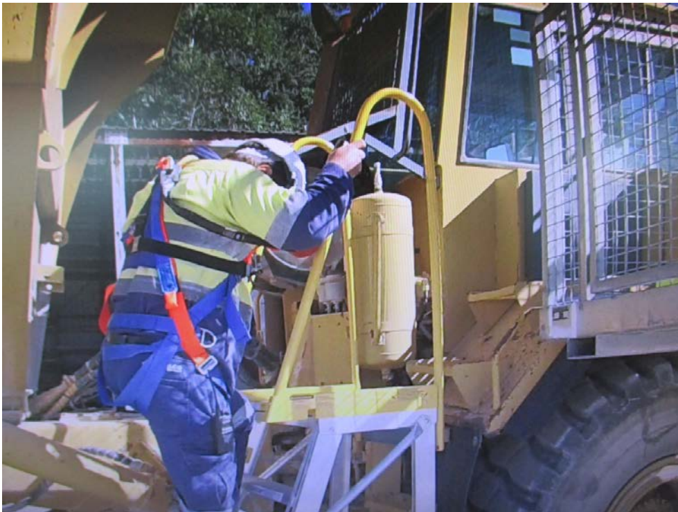
Figure 28: Person descending the mobile ladder using the grab rails to maintain three points of contact.
