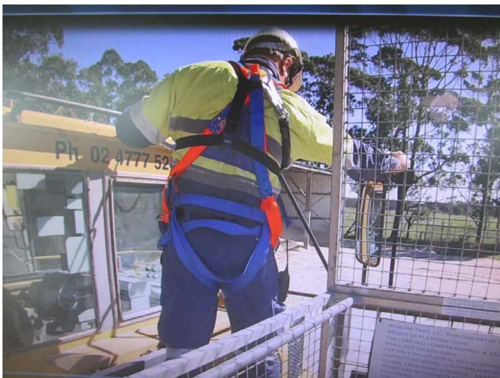
Figure 24: Person opening off-side mirror from platform with mobile edge protection.
