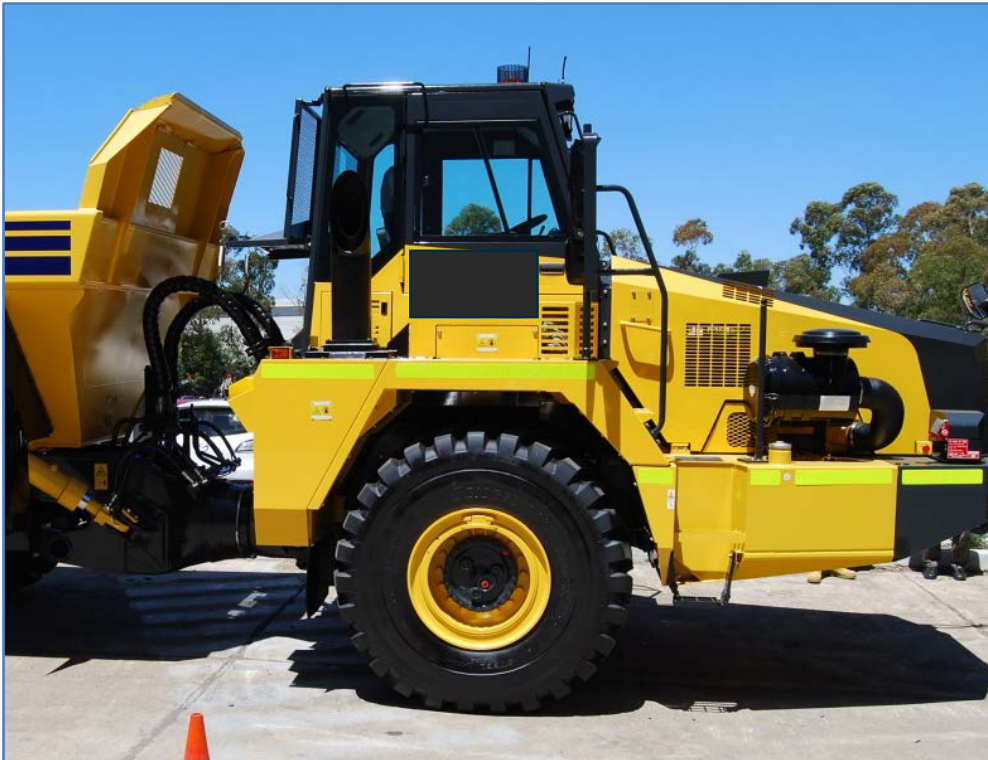
Figure 34: Imported model dump truck without access systems modification.
