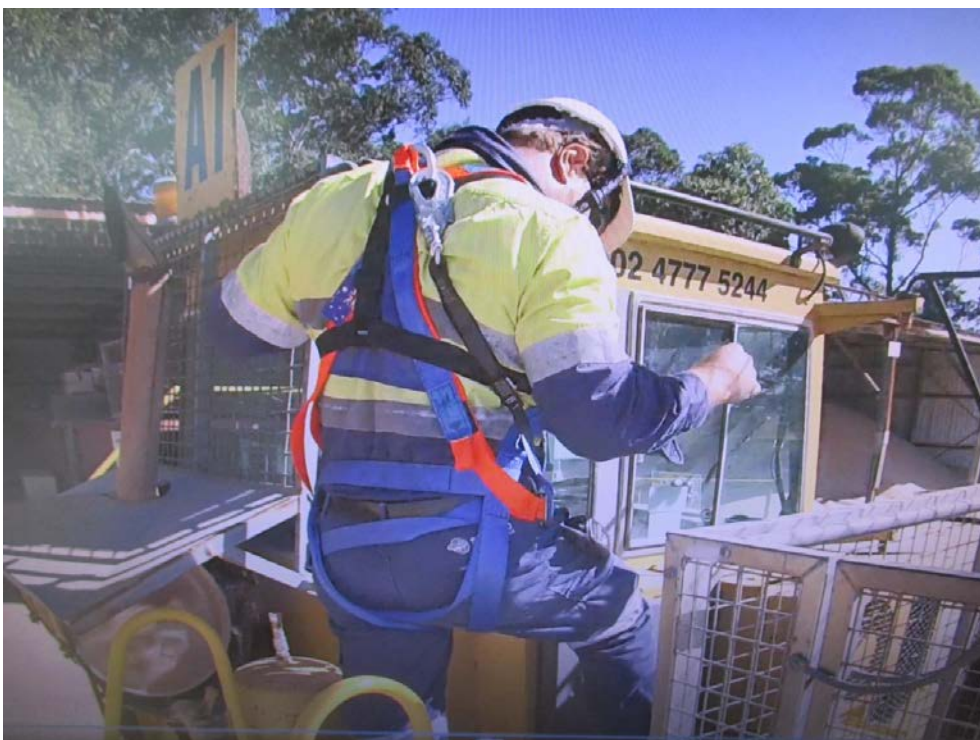
Figure 26: Person on the first stair tread and facing the stair looking for a right hand position to maintain three points of contact as they descend. Three points of contact is possible by first using the outer edge protection provided by the man cage and then the mobile ladder grab rail.
