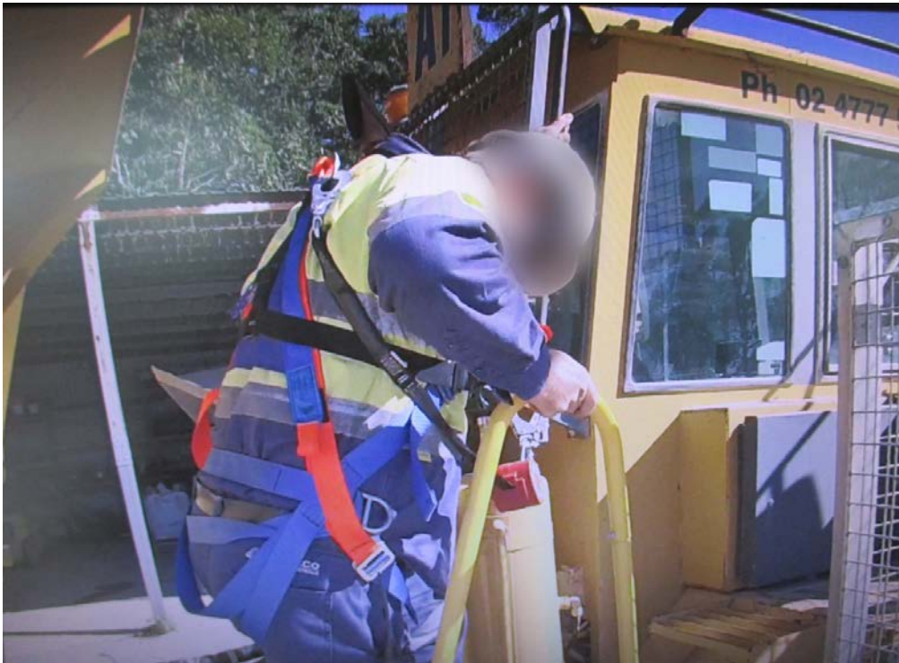
Figure 28: Person descending the mobile ladder using the grab rails to maintain three points of contact.
