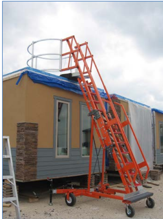
Figure 29: Example of a mobile ladder with fixed edge protection. (Internet photo)
