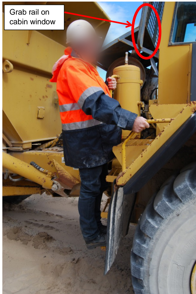
Figure 8: Three points of contact for access onto the first rung of the step ladder.
