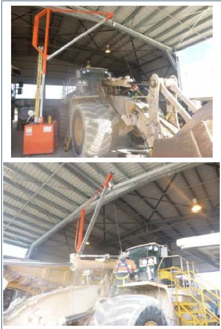
Figure 20: Extract from the Sibelco memorandum dated 23 June 2014, Controls for prevention of falls from vehicles . Shows examples of the use of mobile fall protection equipment when an operator is required to move beyond fixed or mobile guardrails on mobile plant.
