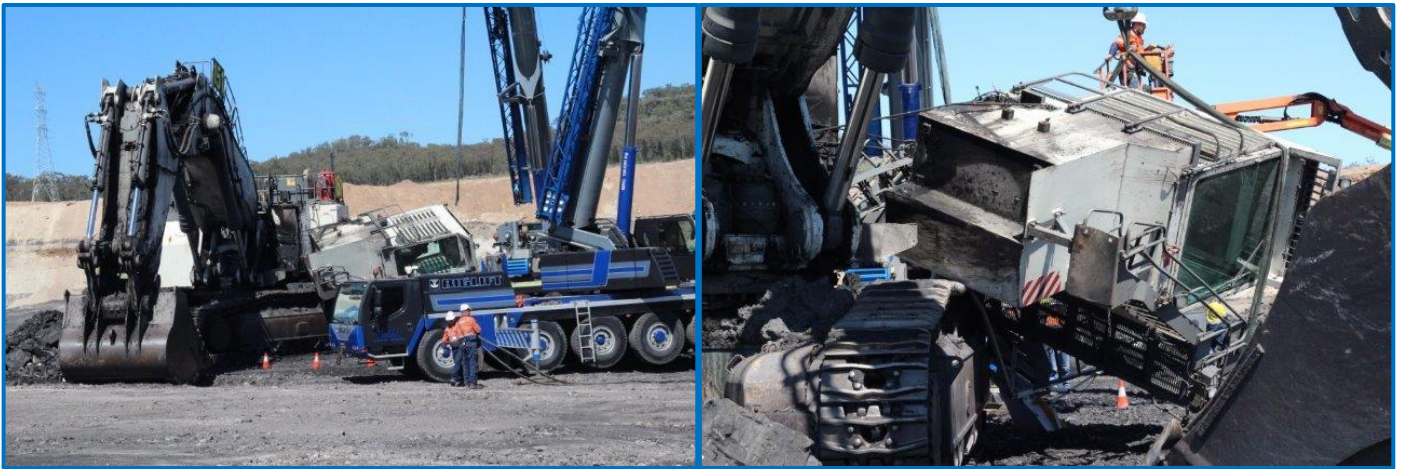
Figure 3: Operator's cabin on the excavator tracks, indicating failed horizontal bolts and interim weld repair.
