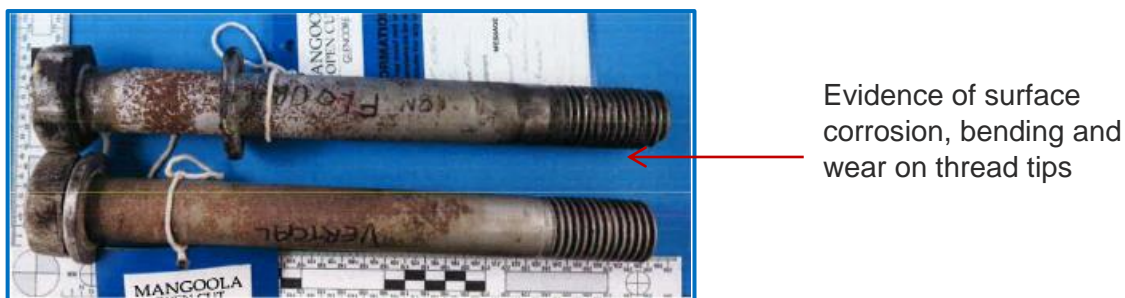
Figure 6: Two broken bolts found at incident scene.
