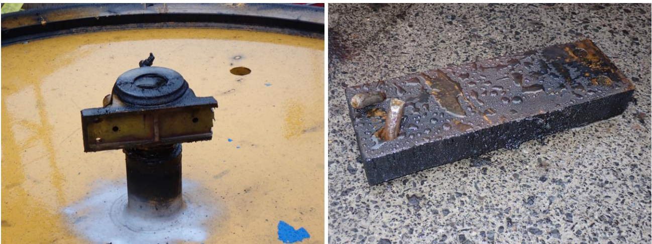
Figure 3 Damaged head sheave pulley wheel assembly components
