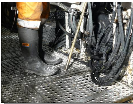
The drill steel and drill bit in the approximate position on the metal plate floor of the mobile bolter.
