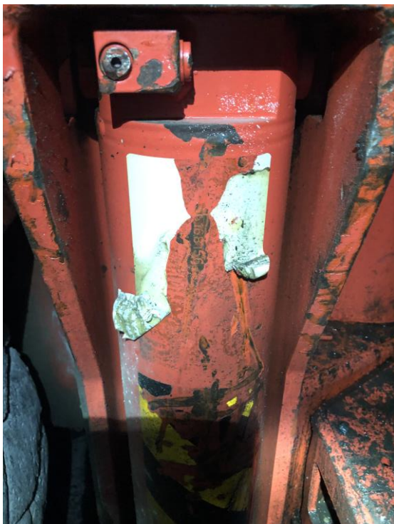
Figure 9. Damaged and illegible warning signage on opposite jack leg
