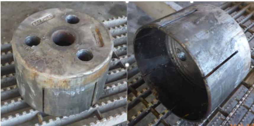
The fitters successfully removed the rear pin outer collet but had difficulty with the front outer collet. They asked that a boilermaker remove the collet by gouging it with an oxy-acetylene torch. A boilermaker performed this task between 7.30am and 10.20am. The fitters tried to extract the pins at 3.20pm, using a hydraulic porta-power and sleeve. Both pins were withdrawn about 70 millimetres, which was the limit of travel for this set of tooling.
