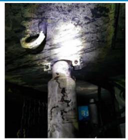
A worker was replacing a leg cylinder on a breaker line support. While positioning to install the top pin, the yield valve
