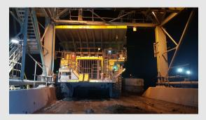
Structures must be protected from impact with mobile plant. The extension of headboards and trays should be considered during the design of barriers and guides. Equipment operators must maintain situational awareness and remain vigilant to manage the risk of collisions while operating mobile plant.
