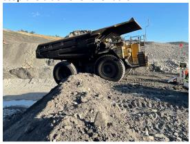
When designing a dump, ground stability should be a primary consideration. Material consistency, wet conditions and dipping ground stability should also be considered. Inspections should verify the dump integrity. Areas that do not meet the standard should be demarcated, communicated and remediated to meet the standard.
