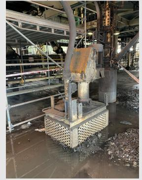
When group isolation systems are used, the isolation must be confirmed for all the required tasks. When workers lock onto a group isolation, they must check that the isolation is suitable for the task they are conducting. Mine workers must be trained and competent in isolation procedures and should always test for dead before starting work.
