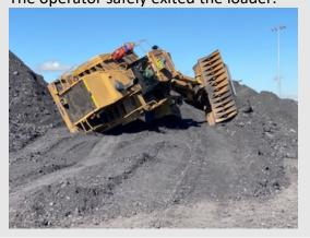
When working on grades and slopes, operators must be cautious when raising implements, such as buckets, and when articulating.
