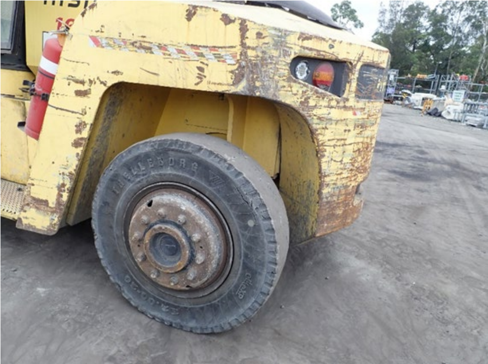
Figure 3 Guarding. Rotating parts contactable through the rear
