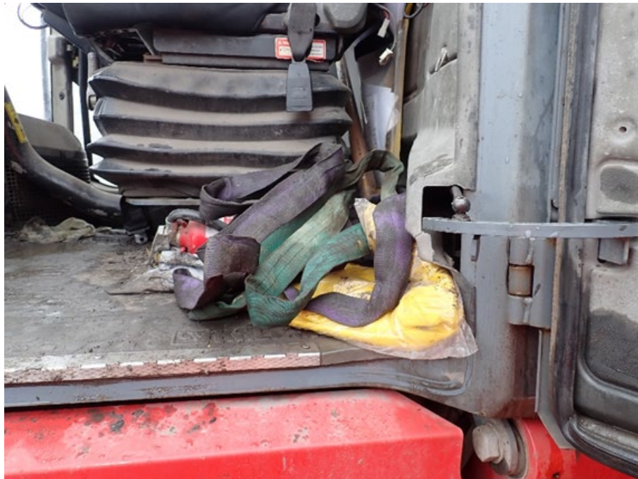
Figure 4 Debris and unsecured items in a forklift cabin
