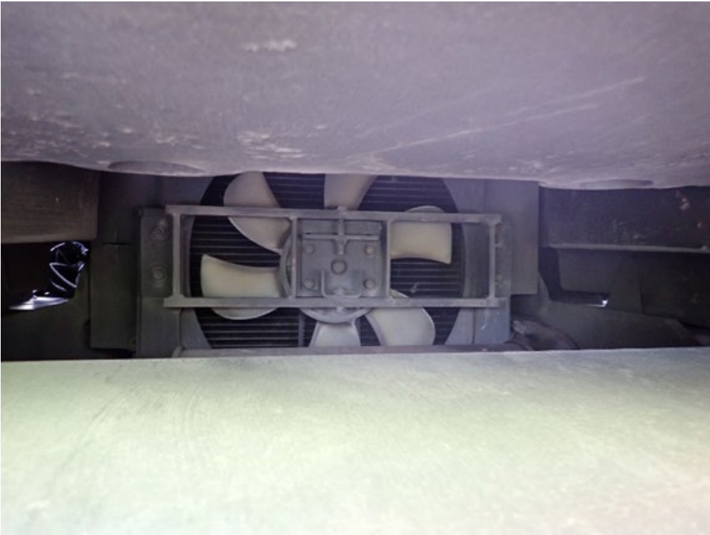
Figure 3 Guarding. Rotating parts contactable through the rear
