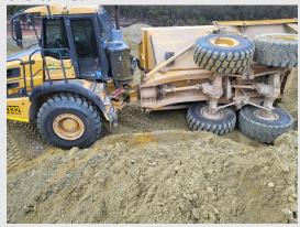
The stability of articulated vehicles is a known risk that needs to be managed at mines. Factors that truck operators must consider include (but are not limited to):
