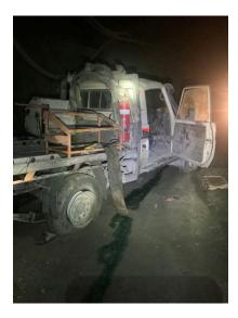
Equipment operators must maintain situational awareness and remain vigilant regarding the risk of machine rollovers. This incident underpins the importance of wearing seatbelts as a mitigating control and demonstrates roll overs can occur in unexpected situations.
