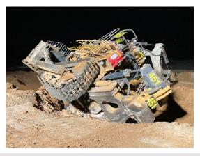
Situational awareness is a key control when operating mobile equipment. Operators should minimise reversing and consider this when planning tasks. Lighting plants should be strategically placed to provide adequate lighting for tasks and reduce glare.
