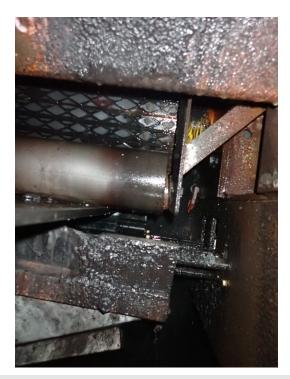
Dangerous incident IncNot0042266 Underground metals mine A fitter was working on a truck while the cab was tilted forward. While working, the fitter bumped the stay, allowing the cab to fall on him. Another worker helped free the fitter from under the cab. The fitter was not injured.
