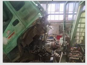
When working under a tilted cab or tray, the support stay must be secured to protect workers from being trapped, pinned or crushed. Stays require a two-step action to ensure they are adequately protected from inadvertent release.
