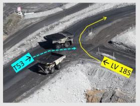
The design of intersection must consider height of windrows and positioning of lights that may affect the visibility of drivers.
