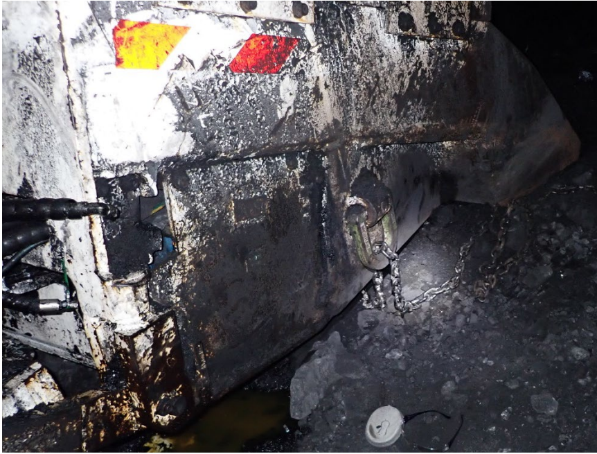
Figure 2 10 mm chain attached to an RUD lug
