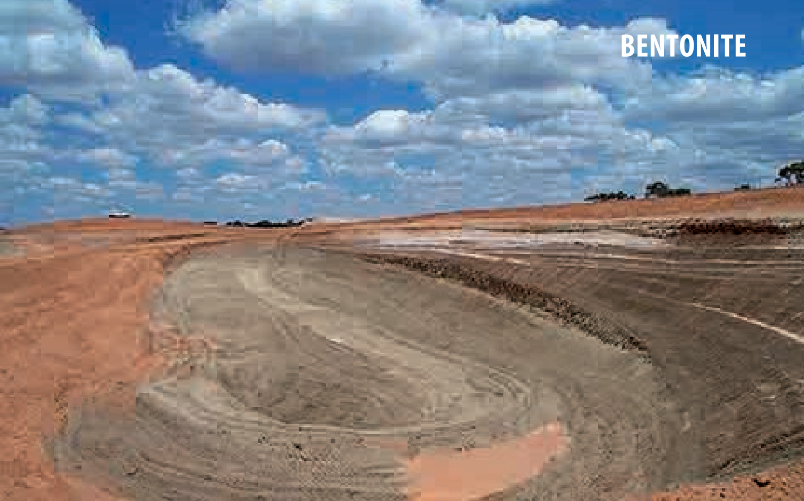
Photograph 2. Arumpo bentonite mine, Arumpo. The bentonite deposit (green–grey clay at base of photograph) contains high-purity sodium–magnesium bentonite formed during the alteration of volcanic ash deposited in the Pliocene Loxton-Parilla Sands. (Photographer J. Whitehouse)
