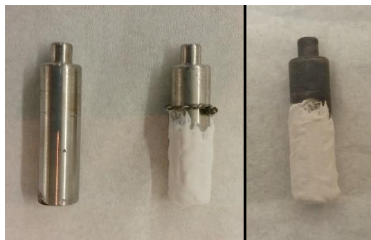
Figure 54: LEFT – Stainless rod before and after painting with Resbond, RIGHT – After heating to 600°C
