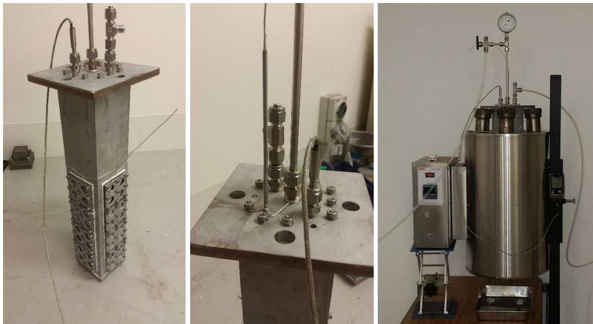
Figure 98: Final assembled cell on bench (LHS) and within vertical tube furnace ready for testing
