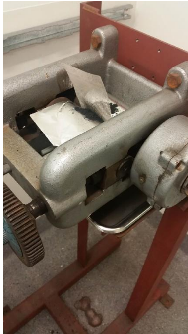
Figure 90: Roller press used for initial anode fabrication investigation
