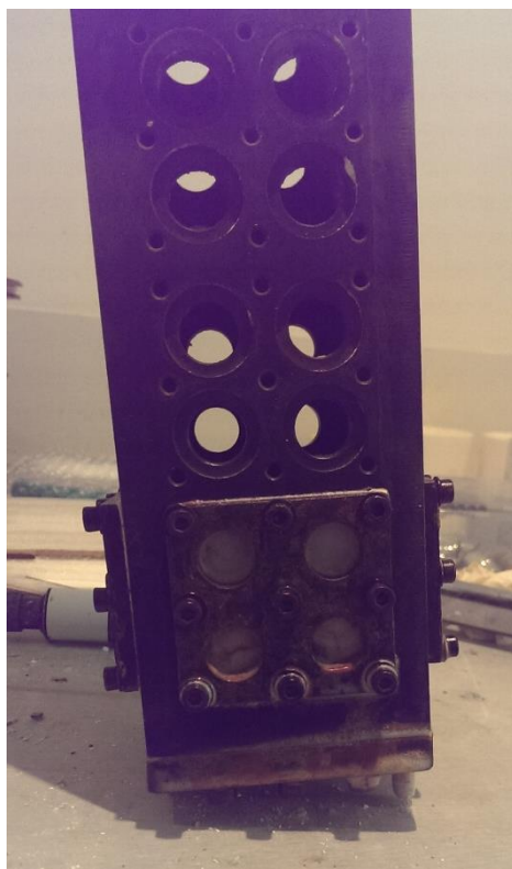
Figure 100. Cell setup used for leak testing.
