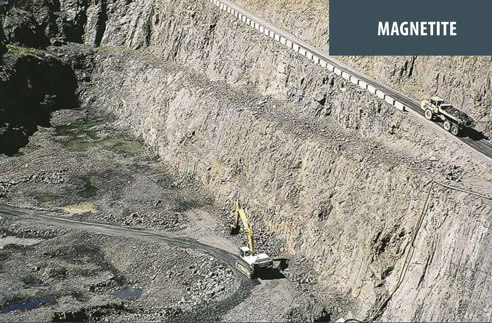
Photograph 15. Tallawang magnetite mine, Gulgong. The Tallawang mine is the sole producer of magnetite in the state. The magnetite is used almost entirely by the New South Wales coal mining industry during coal beneficiation. When finely milled, magnetite remains suspended in water, producing a dense medium suitable for separating impurities from coal. The magnetite is easily recovered by applying a magnetic field. (Photographer I. Paterson)
