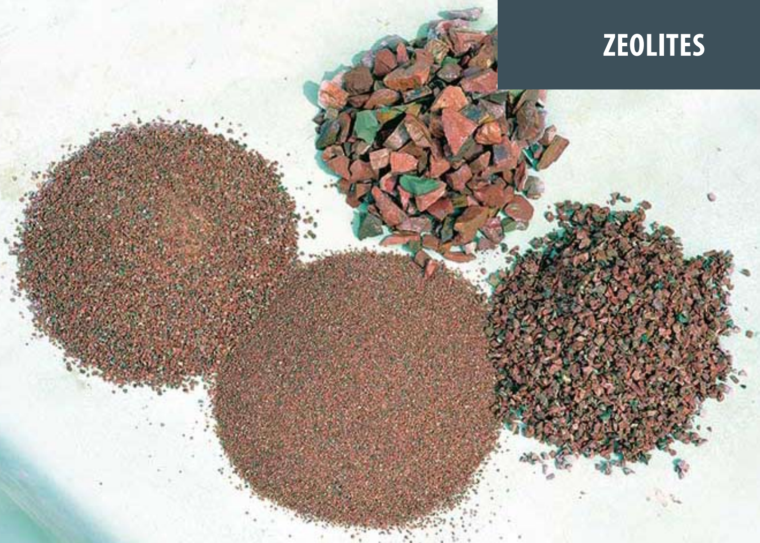
Photograph 25. Crushed zeolite from the Escott zeolite mine, Werris Creek. Zeolite applications include odour control, contaminated site remediation, fertilisers and sewage treatment. New South Wales zeolite deposits are typically high-grade, and much harder than overseas deposits, making them more suitable for such uses as water filtration. (Photographer D. Barnes)
