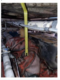
Dangerous incident IncNot0043798 Open cut coal A mechanical tradesperson was undertaking repairs to a large hydraulic excavator. When removing a retaining clamp on the accumulator charge hose, hydraulic oil was Sites must have an energy isolation system in place to identify and control all energy sources for all equipment on
