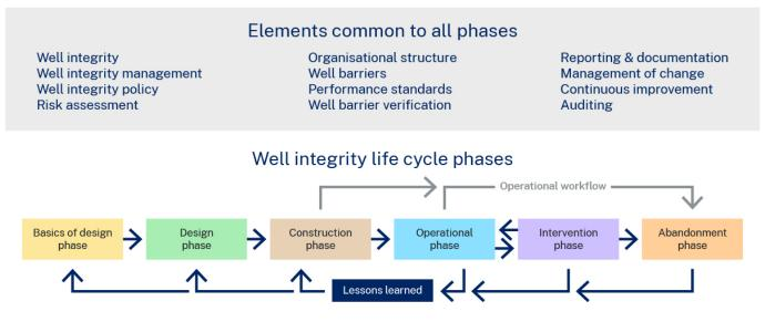
Monitoring and maintenance is required to preserve the well in a suitable condition for its useful life. Well integrity management systems and associated documents for subsurface assets aim to ensure that wells meet operational availability objectives and well integrity goals for the full lifecycle of the well.
