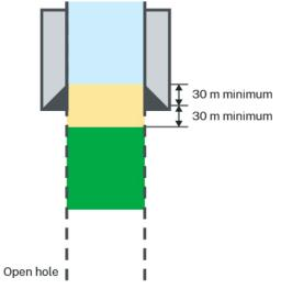
Figure 5: Casing shoe or equivalent with open hole/ uncemented liner below
