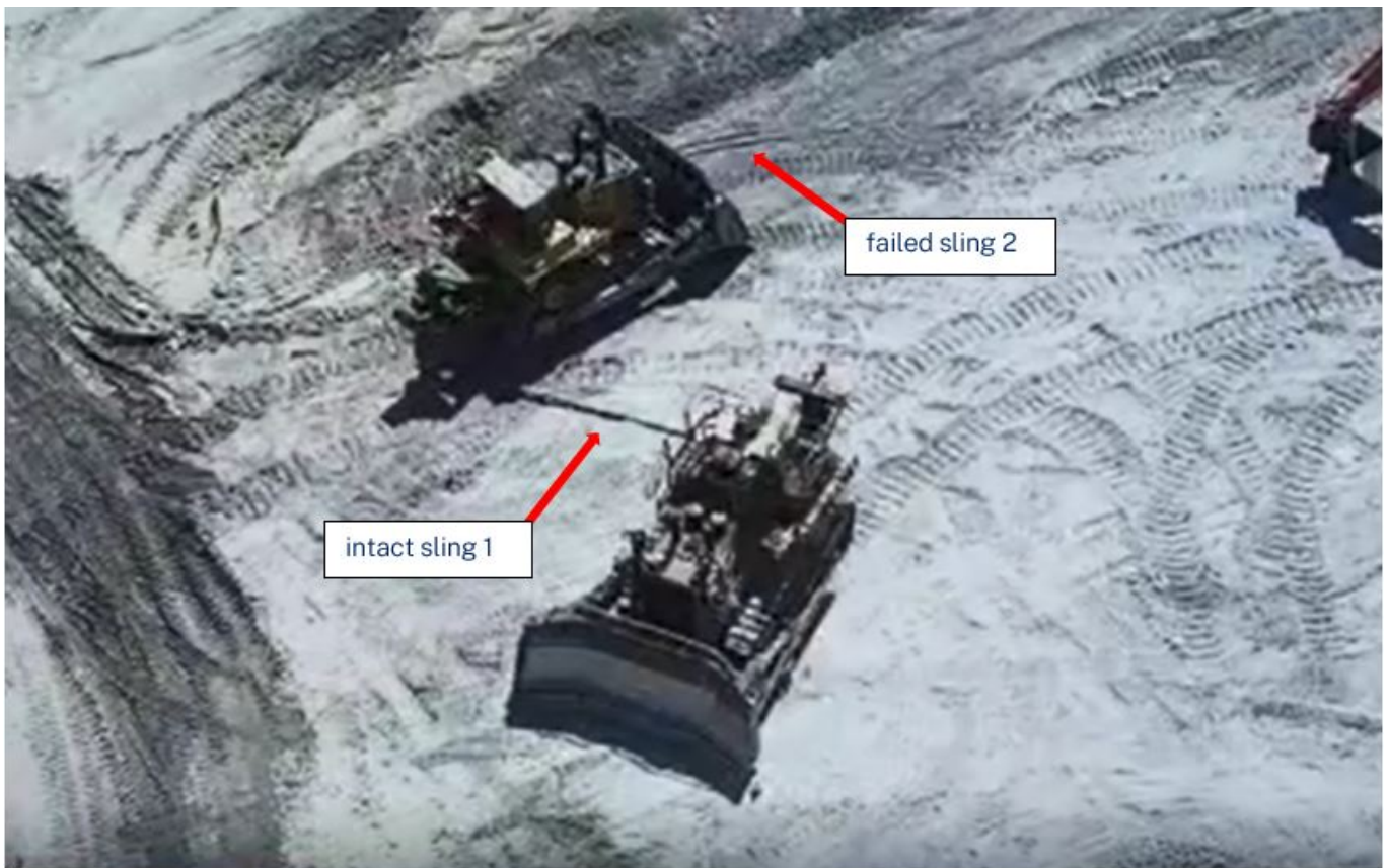
Figure 4: Drone imagery showing the position of the D10 dozer after the rear sling failed
