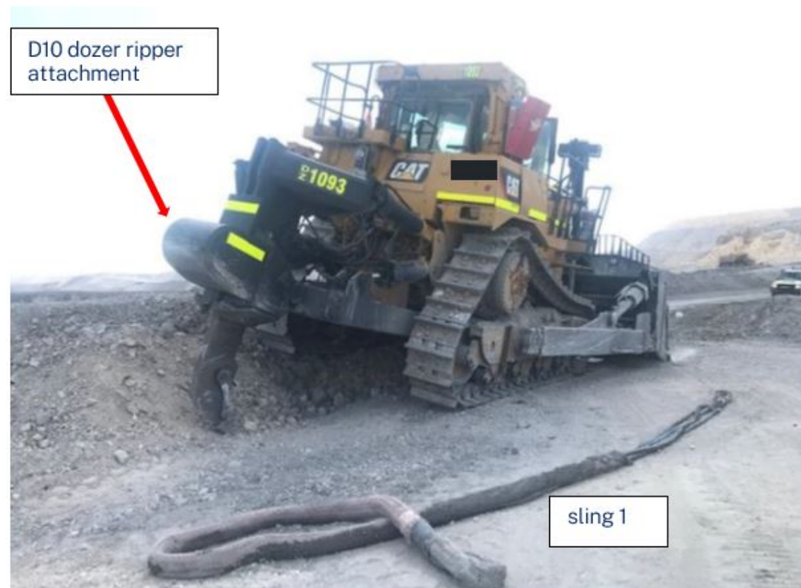
Figure 2: Sling 1 used to connect the ripper attachments of D10 and D11 dozers
