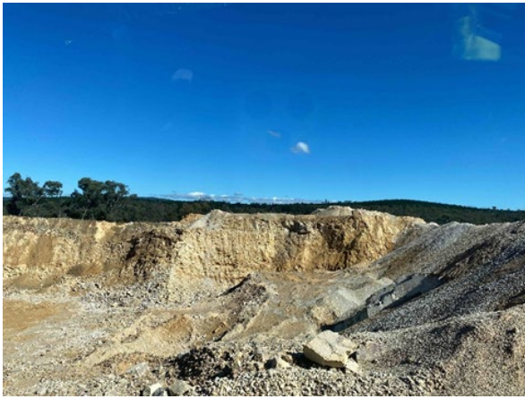
Figure 3 Bund walls around extraction area
