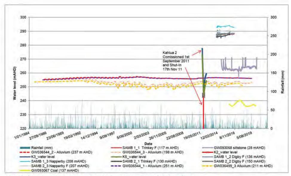
Figure 5.3 Selected groundwater level observation data at, and surrounding, the 2011 Kahlua Pilot test
