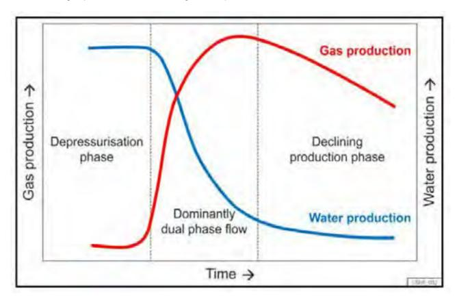
Figure 2.2 Typical gas and water flow profile during CSG production (OGIA, 2021)
