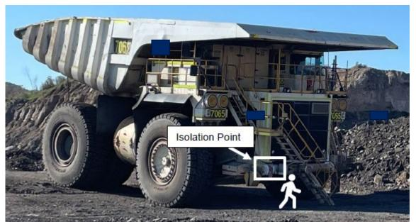
Figure 1: Drawing shows where the truck operator was located when the truck started to roll forward
