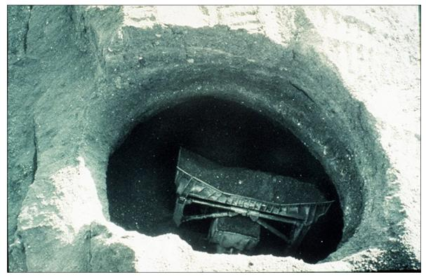
If the windows of the stockpile dozer cab are not designed to withstand the burial forces applied, material can flow into the dozer operator's cab, placing the dozer operator at risk of engulfment, suffocation, and death.
