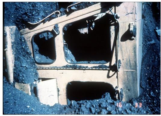
For coal stockpiles there is a potential for coal to ignite if in contact with heated surfaces of the dozer.
