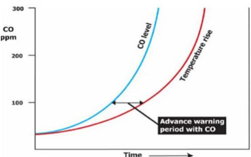
Figure 7: Ventilation airflow Fire advanced warning - CO vs. temperature
