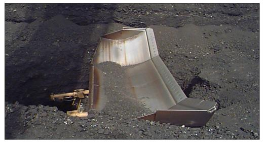
Parking up stockpile dozers and other plant adjacent to the draw point (within a high-risk zone) is hazardous. The plant or vehicle's parking position is particularly important. For example, the hazard is greater if the position is of least stable alignment to, and potentially within, the area of influence of a draw point.
