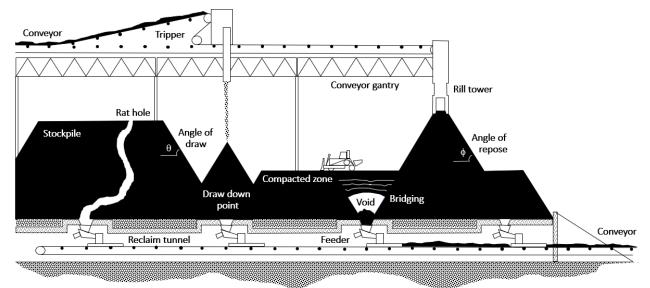
Where a stockpile base and surface are not graded to allow water run-off and prevent the formation of central reservoirs, water may accumulate in a partially extracted stockpile. This can happen when a stockpile base and surface are not graded to allow water run-off and prevent the formation of central reservoirs. Water collection sites can sometimes only be discharged through the draw point. See section 4.1.7 Flooding for further detail.
