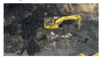
When working under benches and walls, a safe stand-off distance should be defined, communicated with workers and maintained throughout the task.
