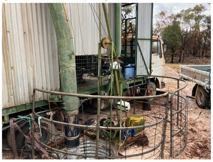
Figure 2: Cable from hoists drum was found completely unspooled
