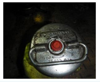
Mine operators should inspect all coolant systems to ensure warnings are in place and a means is available to dissipate the stored pressure to protect workers from exposure to hot coolant. Each radiator filler and radiator cap should be arranged or interlocked so that coolant pressure is safely released prior to the cap being able to be removed.
