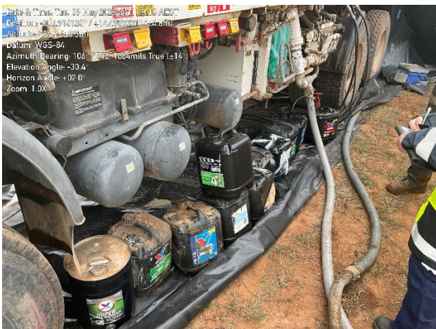
Figure 2 Oil and chemical storage on the rig nappy underneath the drill rig
