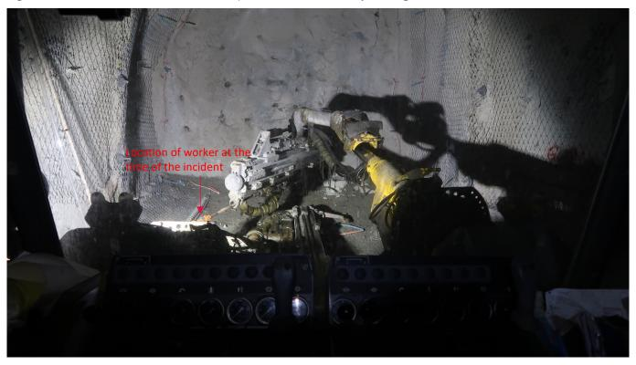
Figure 3: Drill steel inserted into coupling on the righthand drill
