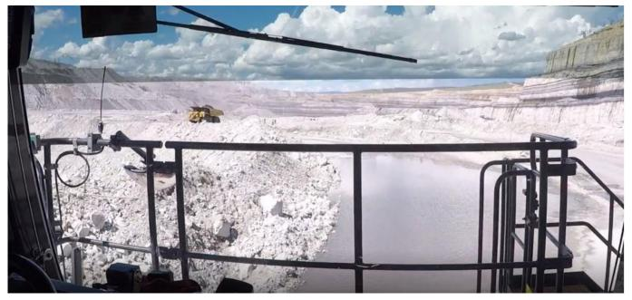
Testing conducted as part of the investigation identified the light vehicle became partially visible to the haul truck operator when he was about 88 metres away from it. However, as can be seen by Figure 7, it is difficult to identify the light vehicle even with the benefit of hindsight. Additionally, the presence of the Caterpillar truck at the intersection (and other distractions referred to in Section 4.1.5) drew the haul truck operator's attention away from the light vehicle.
