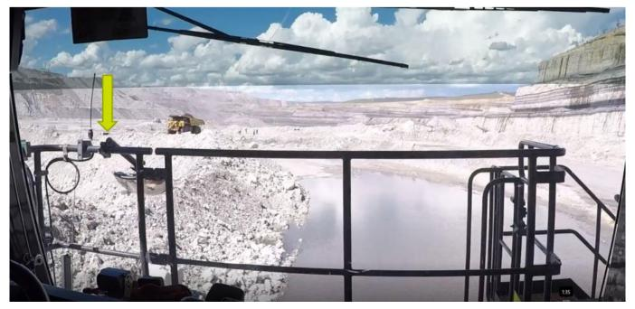
As the haul truck continued to travel along the road approaching the intersection, the light vehicle continued to be fully or partially obscured by the windrow as shown by Figure 8 and Figure 9.
