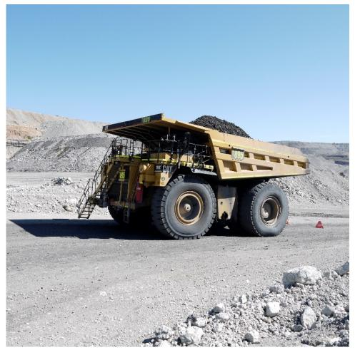
This may have impaired the operator's ability to see the light vehicle by changing the angle of his field of view, effectively increasing the size of the truck's height related blind spot.
