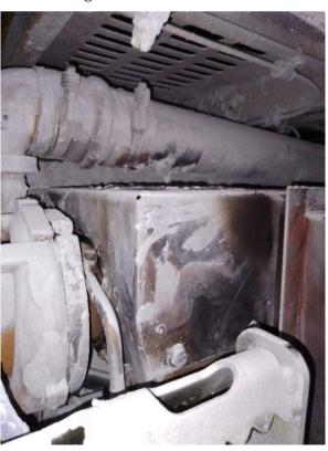
The failure of oil and fuel lines near exhausts and turbochargers are well-known causes of fire. Fuel sources and ignition points should be separated or have other controls in place to prevent fires.
