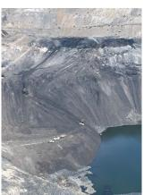
Mine operators should review and update their dozer bulk push risk assessment and associated procedures to include the requirement to clearly define the dozer bulk push area to prevent dozers from working in areas of risk.
