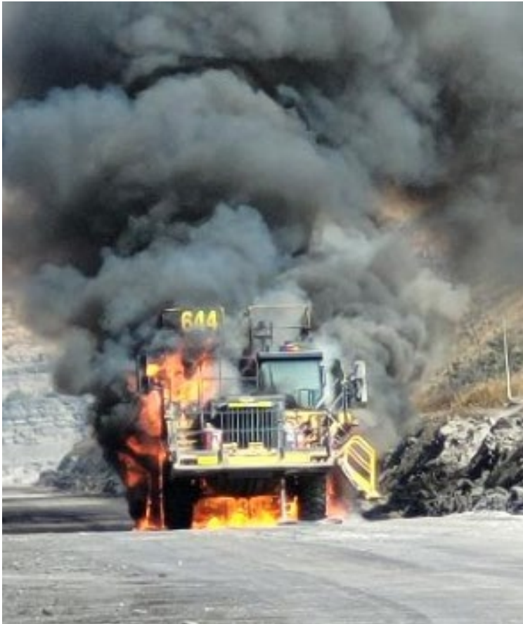
Figure 3: Caterpillar 773F service cart fire
