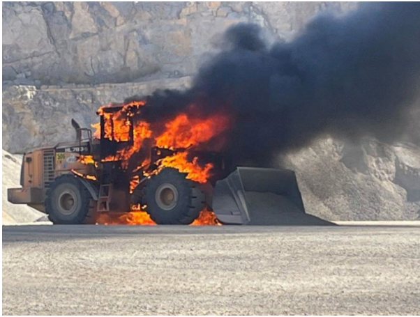
Figure 1: Hyundai 780-9HL loader fire
