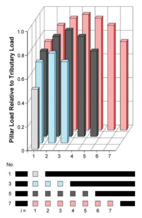
Figure 6 - An example of the influence of panel width on pillar  $\mathsf{load}^{17}$
