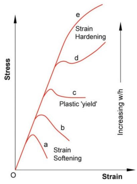
Figure 8 above shows the way that pillar width-to-height ratio influences its behaviour. After a pillar with a low width-to-height ration exceeds its maximum resistance to deformation, it undergoes strain softening and progressively and permanently unloads with ongoing displacement. This is depicted by curve (a).
