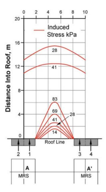
The example analysis in Figure 13 predicts that the units generate more than 40 kN (4 t) of upward force per square metre some 12 m up into roof between the midpoint of the pairs of MRS.
