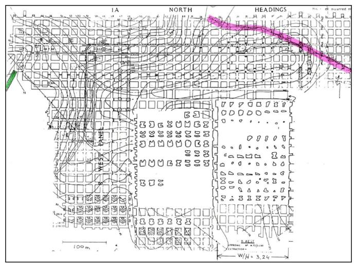
Figure 30 – Mine plan showing area involved in pillar instability event at Awaba Colliery<sup>52</sup>
