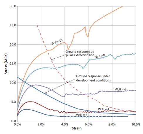
The modelling predicts that pillars with a width-to-height ratio of 8 would be in a pre-peak stress state under development conditions. Post-peak yielding occurs as the extraction line approaches and the pillars are loaded beyond their initial peak. At these relatively high stress values, the ground response is stiff, and equilibrium is reached at a vertical strain value of 3.2%.
