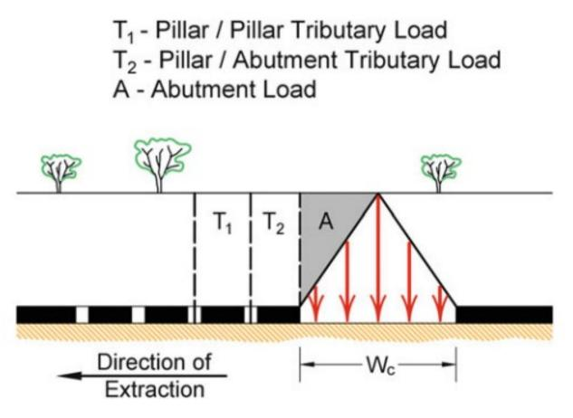
Bridging superincumbent strata can adversely affect pillar extraction operations because it increases abutment stress and the propensity for windblast and gas inrush<sup>23</sup>.
