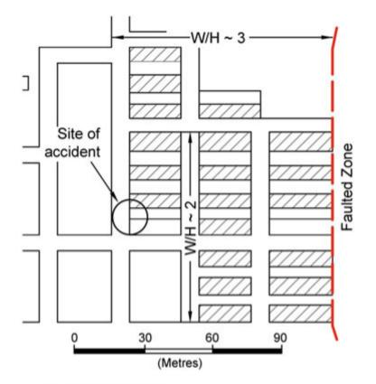
Mining height 2.4m. Depth 20-30m. Standing goaf > 60x90m. Therefore minimum W/H>2. No rib spall, roof sag, floor heave or observable deflection of props prior to fall. Mass vertical movement to surface. Windblast. Conditions excellent around edge after fall.
