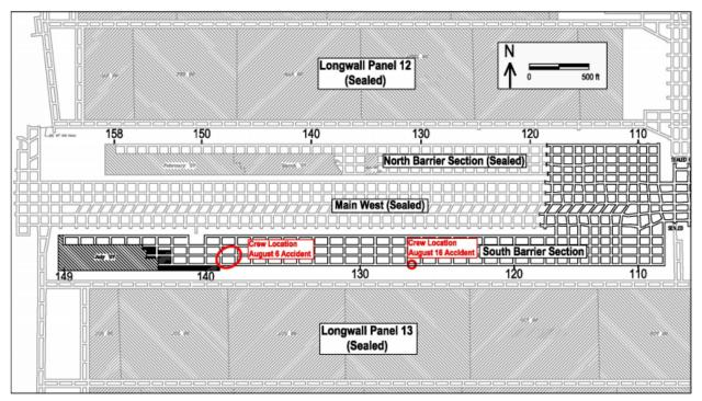
Figure 35 - South Barrier Section Rescue Area Showing Ground Conditions and Rescue Attempts<sup>61</sup>
