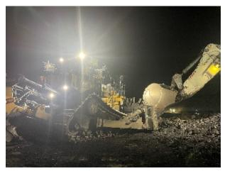
Dozer drivers should maintain a sufficient buffer between their machine and the swing radius of an operating excavator.
