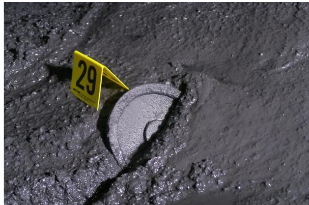
Figure 5: 150mm shouldered galvanised coupling
