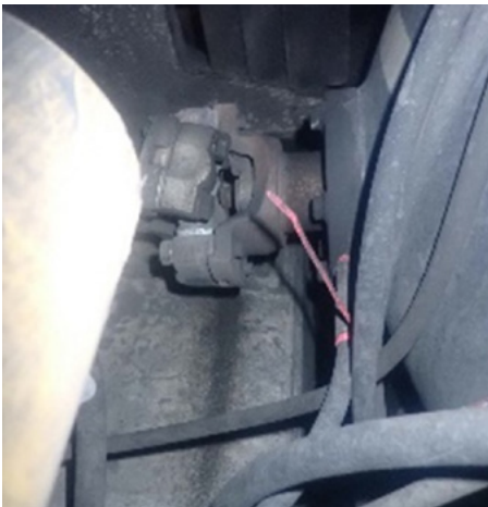
Picture 19. Damage from engine bay fire on LHD.
