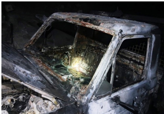
Picture 16. Damage to light vehicle from fire.
