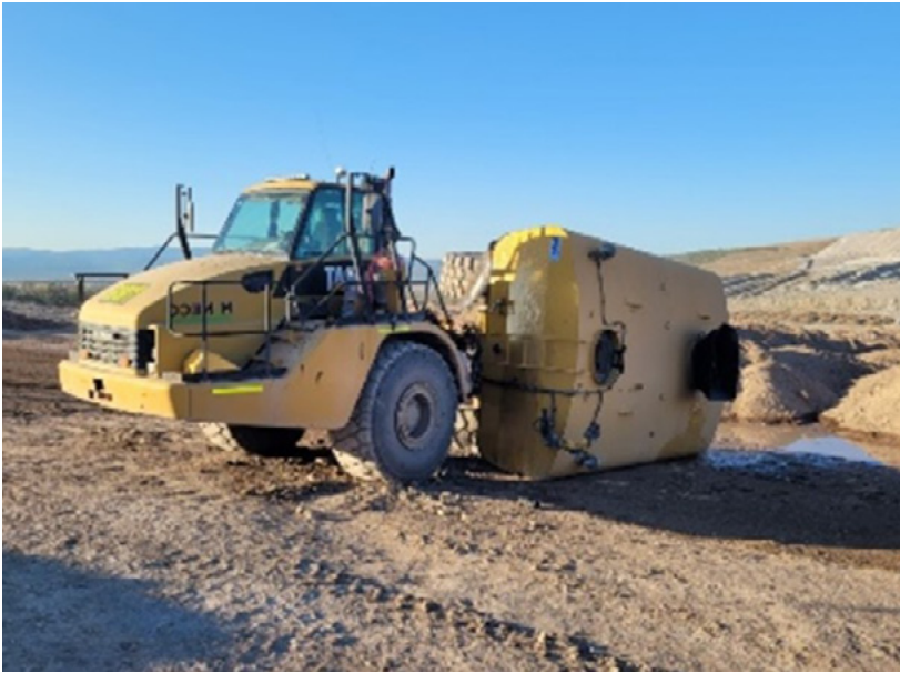
Picture 12. Overturned body of articulated water cart truck.
