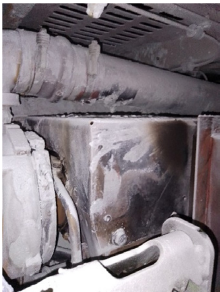
Picture 20. Damage from water cart engine bay fire.
