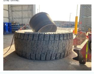
The dangers associated with tyre handling are well understood and mine operators should ensure that their procedures have identified the risk of uncontrolled ejection of a rim from a tyre, and that appropriate controls are in place to manage the risk.
