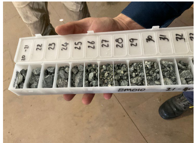
Figure 8 Typical chip sample storage in plastic chip trays with labelling
