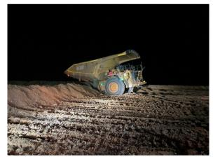
Windrow design, construction and maintenance is a critical factor in dump safety. Mine operators should:
