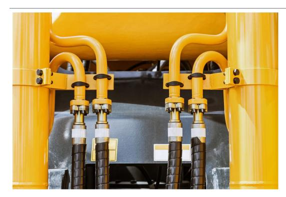
Spiral wrapping prevents rubbing wear and good clamping segregates hoses
