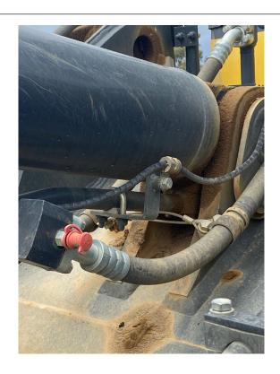
Whip check prevents failed hoses from flailing near operators
