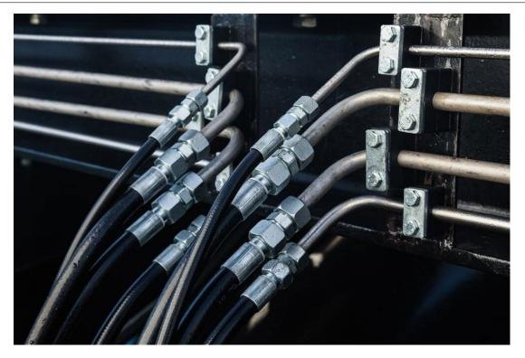
Good clamping keeps hoses segregated. NO cable ties
